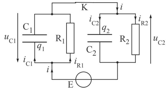
•  $\textcircled{2} \xrightarrow{\textcircled{3}} i = \frac{1}{R_2 C_2} \left( C_2 E - \frac{C_2}{C_1} q_1 \right) + \frac{d}{dt} \left( C_2 E - \frac{C_2}{C_1} q_1 \right)$
